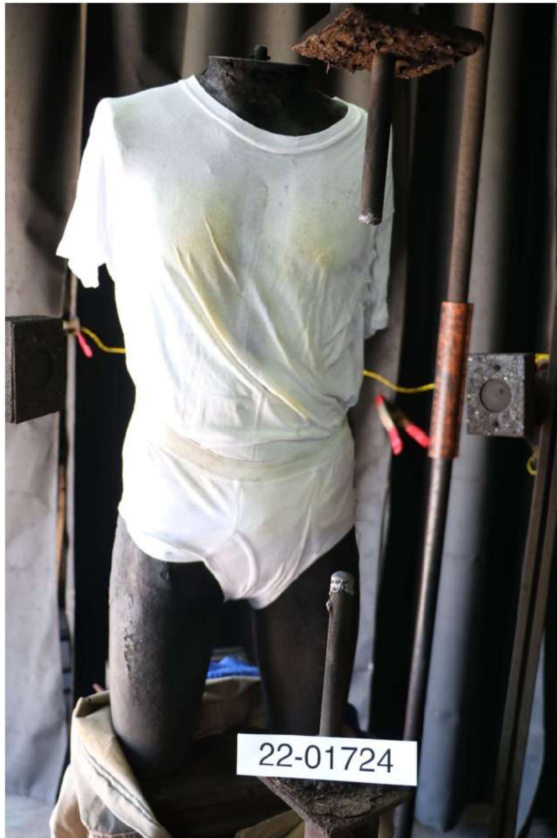
Figure 6.3: Undergarment after arc exposure. (Test# 22-1724)
