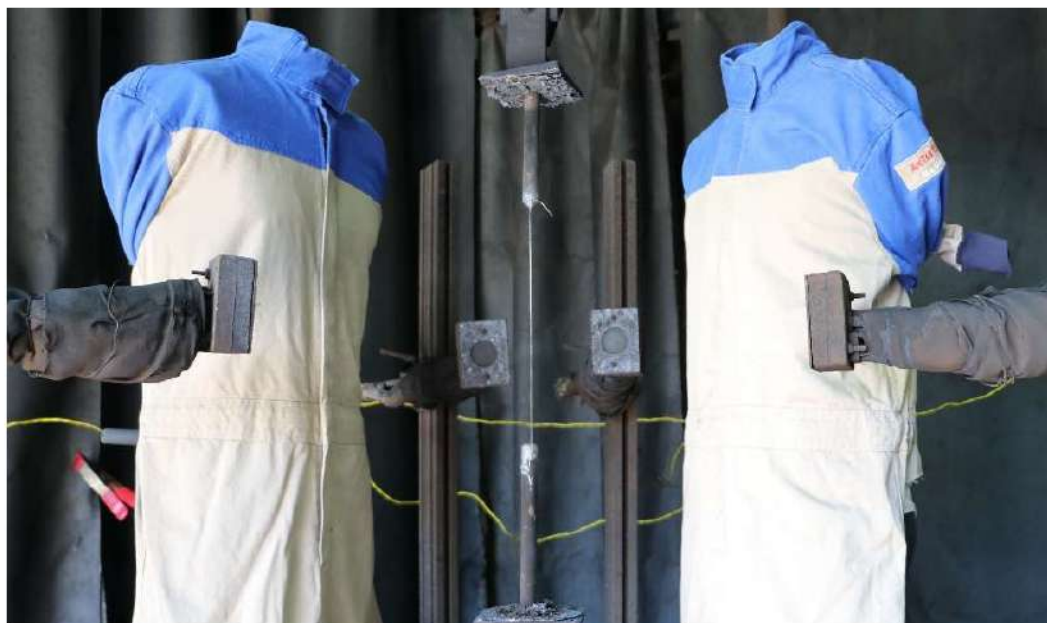
Figure 6.1: Garments as tested before arc exposure.
