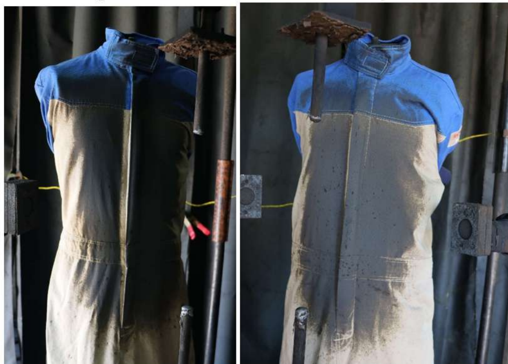
Figure 6.2: Garments after arc exposure. (Test# 22-1724)
