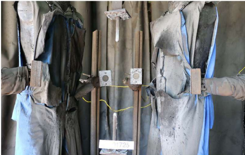
Figure 6.2: Garments after arc exposure. (Test# 22-1725)
