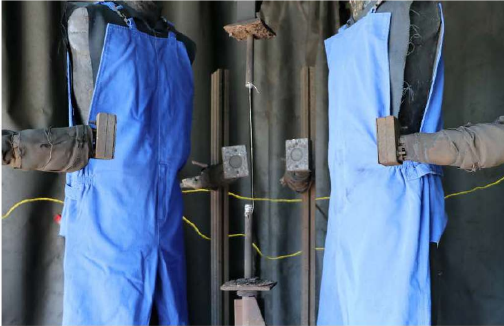
Figure 6.1: Garments as tested before arc exposure.
