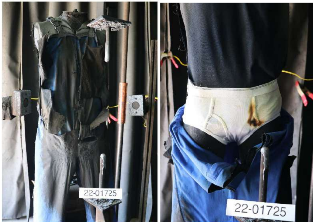
Figure 6.3: Exposure of garment and underlayer garment. (Test# 22-1725A)
